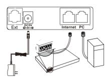
Note: If Power over Ethernet is being used, do not plug in the AC adapter.
